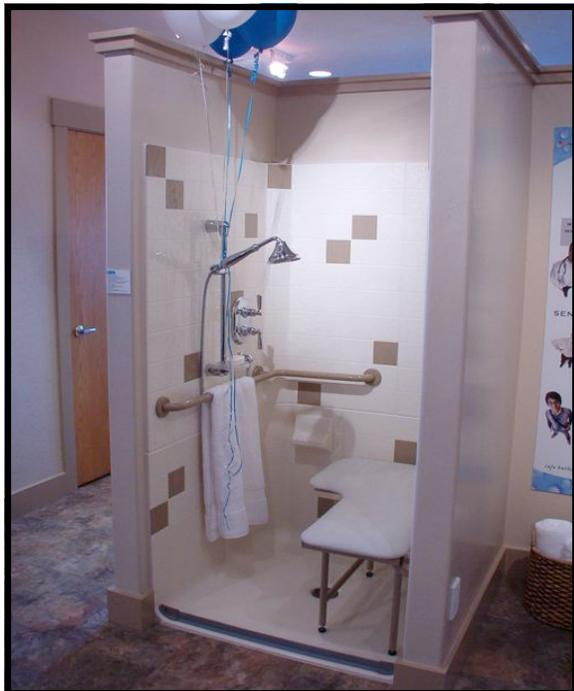
*A 4 piece shower with barrier free curb, seat, and grab bars installed on accented walls*
